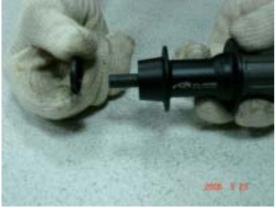
Step 8 Replace the outer washer seal to the hub shell side
