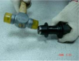
Step 3 Using the soft side of the rubber mallet, gently tap the bearing into the hub shell until it is properly seated in the hub shell (see photo 3.1)
