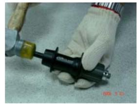
Step 2 Using a rubber mallet, strike the left side of the axle, removing the axle from the hub shell (see photo 2, 2.1)
