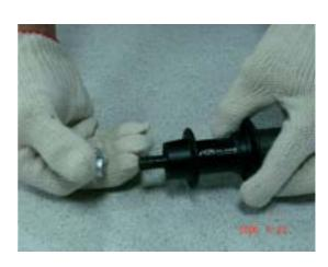
Step 1 Using a 2mm allen wrench, loosen the axle cap on both sides of the hub and remove the end caps (see photos ' 1, 1.1, 1.2)
