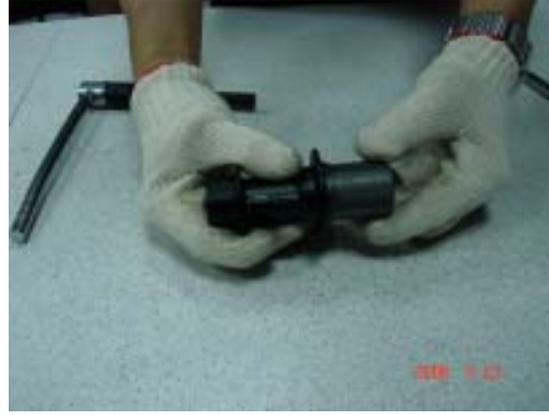
Using the same 12mm & 7/16 " allen wrenches insert them into the hub. Tighten the nut to 500-600 kgf/cm (see photo 1.1, 1.2, 1.3)
